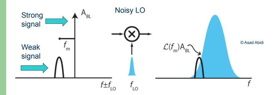
Noisy local oscillator (LO) transfers its noise to the strong out-of-passband signal and on top of the weak signal we are trying to copy.
